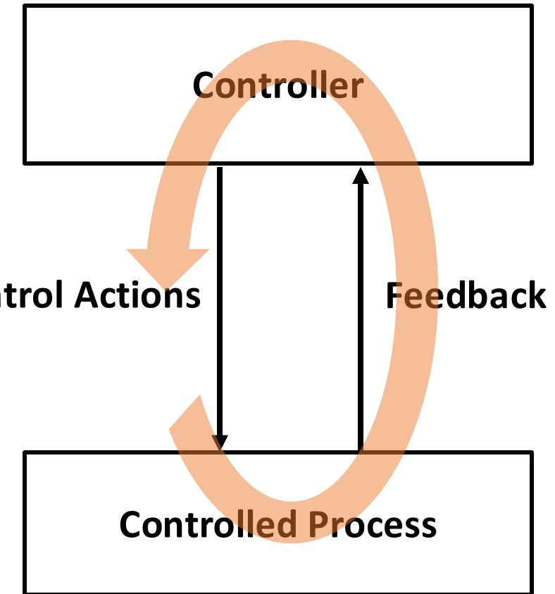
**Systems Theoretic Process Analysis\* (STPA) analyzes the control loops in a system to identify how unsafe behavior could occur**
