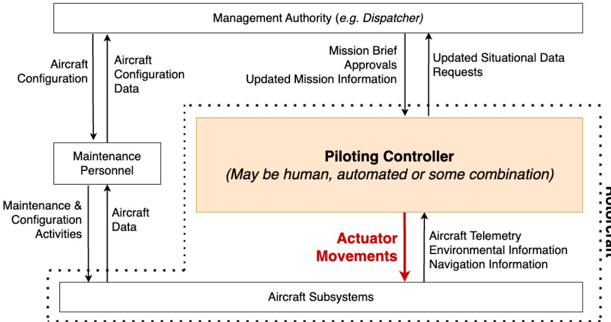
**Example Unsafe Control Action:** Piloting controller provides actuator movements that steer the aircraft toward another aircraft or object
